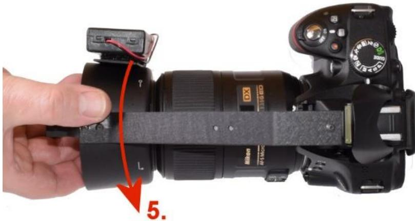
9. Rotate focus light power control clockwise to switch it on:
