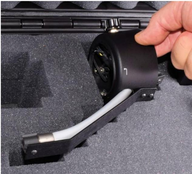
4. Remove lens cap and **turn the camera on.**
