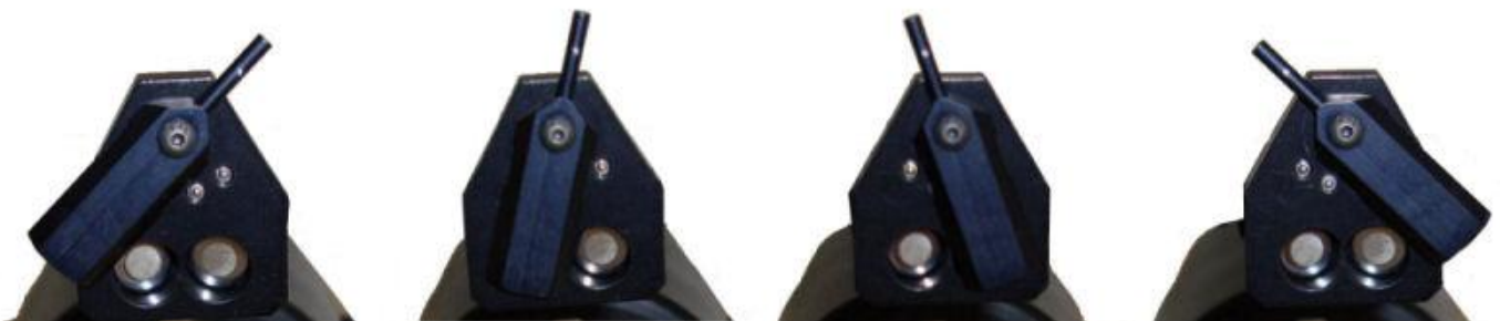
Close-up view of the lightguide shutter in 4 positions:
