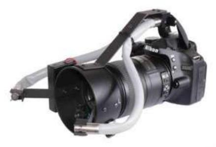
In most cases, the FSL (Fixed Side-Lighting) is recommended – it tends to result in less glare with the brown iris and is super easy to use.
